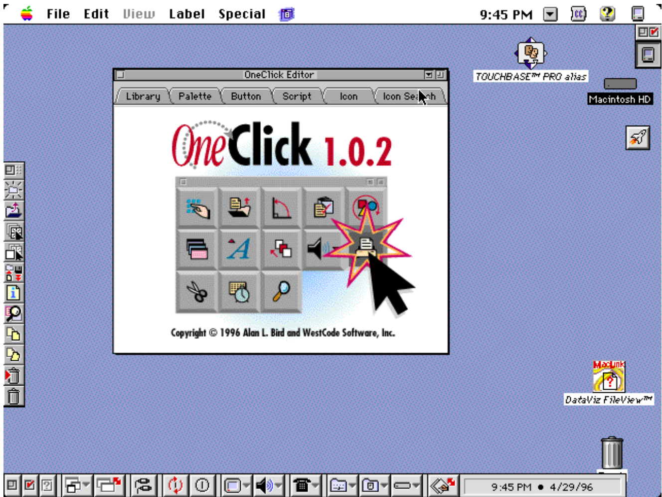
Figure 1. This screen snapshot shows the Finder palette on the left, the System Bar palette on the bottom, and the Task Bar on the upper right. The Launcher has been iconified into a small button with a rocket icon.
